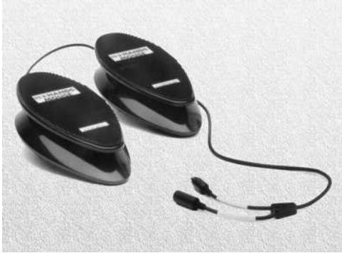
Image 2: NoHands Mouse (left) and Foot-Switch (right)
