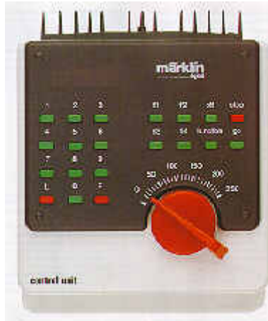
Image 1: Märklin Digital 6021 Control Unit Interface
